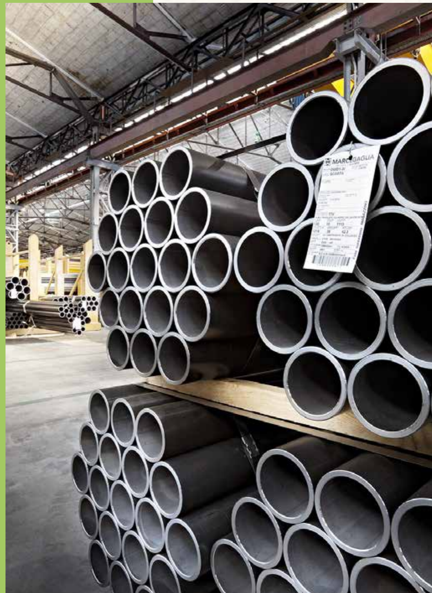
Tube sections from hot and cold strips, heat treated and drawn
